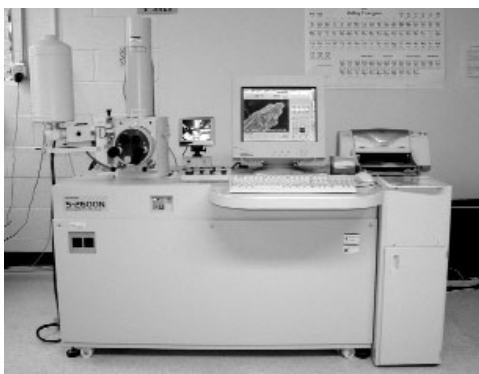
Figure 1. SEM acquired by the Survey early in 2003. The microscope is equipped to perform energy-dispersive X-ray microanalyses.
