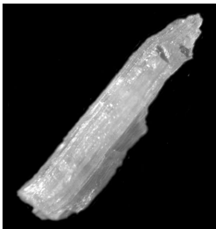
Figure 2. Optical photomicrograph of the celestine sample selected to illustrate the uses of the SEM. The sample is 3 mm long.
